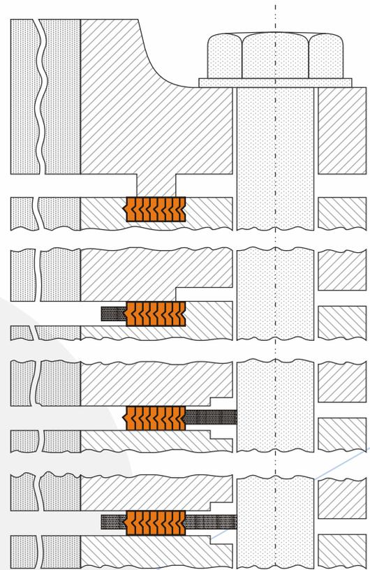
Champion Metallic Gaskets are made as per ASME B16.20 to suit ASME B16.5 flanges and as per "A" Series and "B" Series to suit ASME B16.47 flanges. We can offer on request CMG as per DIN 2632-2638 , IS Standards also .
