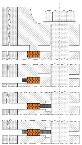
Champion Metallic Gaskets are made as per ASME B16.20 to suit ASME B16.5 flanges and as per "A" Series and "B" Series to suit ASME B16.47 flanges. We can offer on request CMG as per DIN 2632-2638, IS Standards also.
