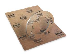
Champion Style 11 is a Economical Grade Compressed Fibre Jointing used for general purpose applications like steam, water, gas, light acids and alkalies. Its constantly uniform solid run constructed using fibres vulcanized with elastomers to develop a dependable performance sealing product
